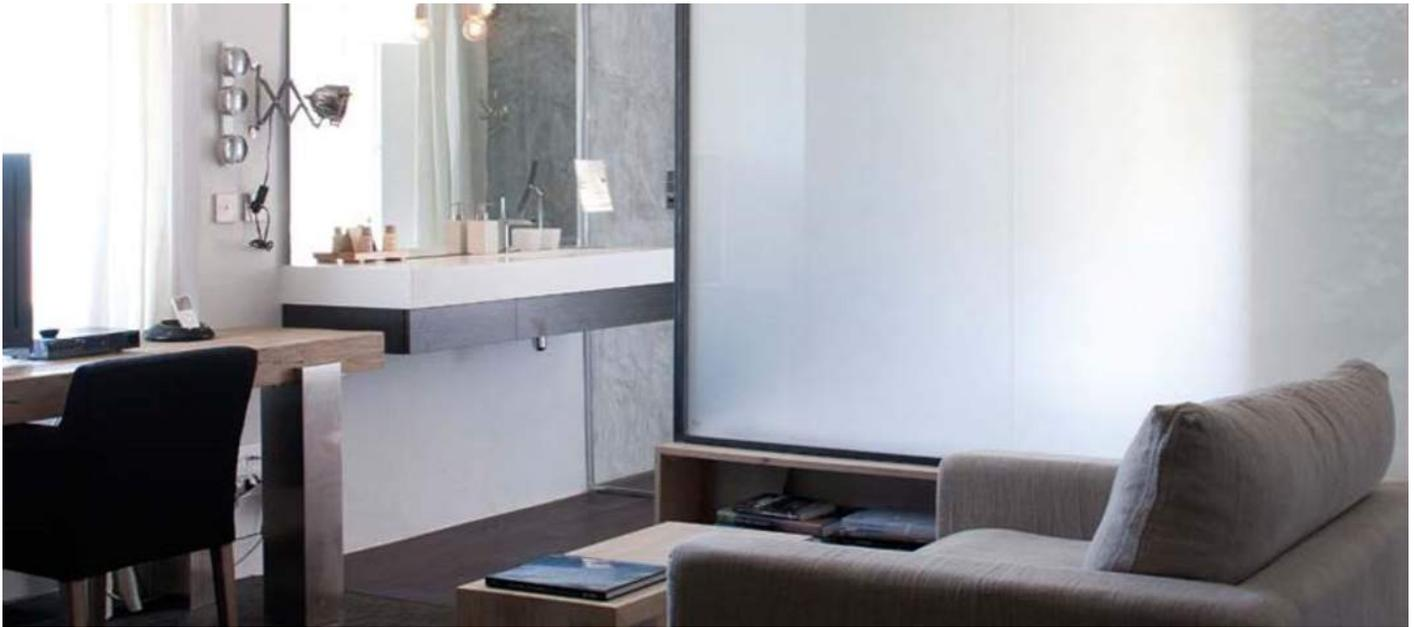
Privacy Glass is an electronically switchable glass solution that allows manageable privacy and vision through glazing whilst maintaining high levels of light transmission.
