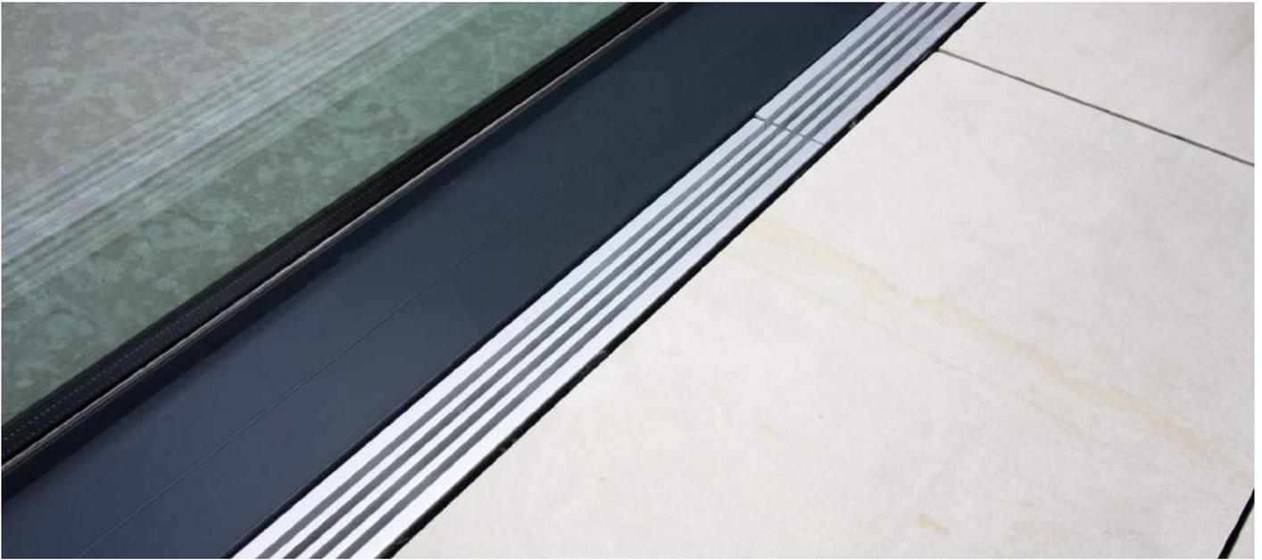
The IQ Flush Drainage channel provides a robust and effective water protection and drainage for flush threshold base frame details. The hidden drainage channel can take up to 90 litres of water per minute.
